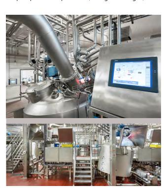
MULTICOOK processing vessels can be operated in semi-automatic or in fully automatic mode. All important processing parameters such as: cooking times, mixing, homogenizing, temperatures and vacuum level are controlled and can be regulated. Recipe management and process flow can also be automated
